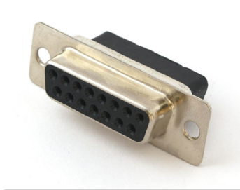
Figure 14-6. Hall and Encoder Mating Connector
