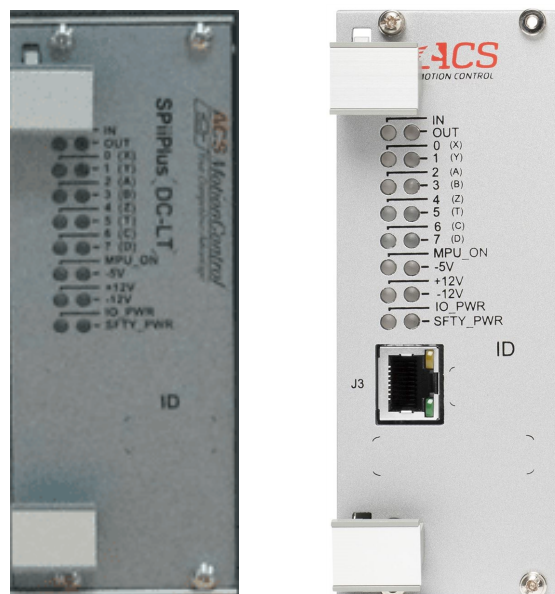
Figure 2-22. Control module without and with the secondary EtherCAT port
